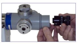
8420 AlignCam eyepiece removal.
