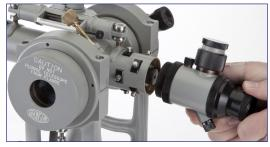
8440 AlignCam eyepiece removal.
