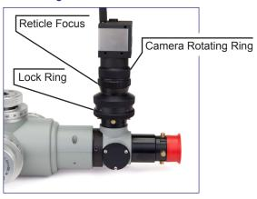
If the Lock Ring is in the way, rotate it CW until it seats against the adapter body to allow full travel of the Reticle Focus ring. The images on the previous page illustrates the camera adapter adjustments.
