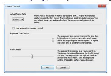
the frame rate and exposure time to achieve a proper image.
