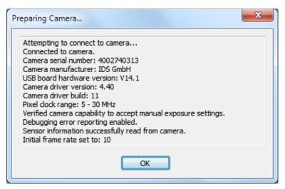
The camera may be disconnected or reconnected at any time, the software simply reconnects when the camera is available.
